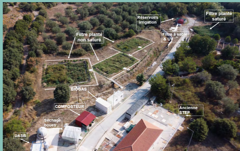
Layout of the wastewater treatment system
